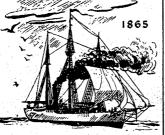
in ocean vessels, captains insisted on sails, too. At first, ships had paddle wheels at the side, later propellers came into use
